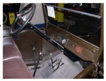
verse. Holding the left pedal half-way down and pressing the reverse pedal, backs the car up. The right-hand pedal is the brake. Levers on the steering column are spark advance on the left and throttle on the right.
